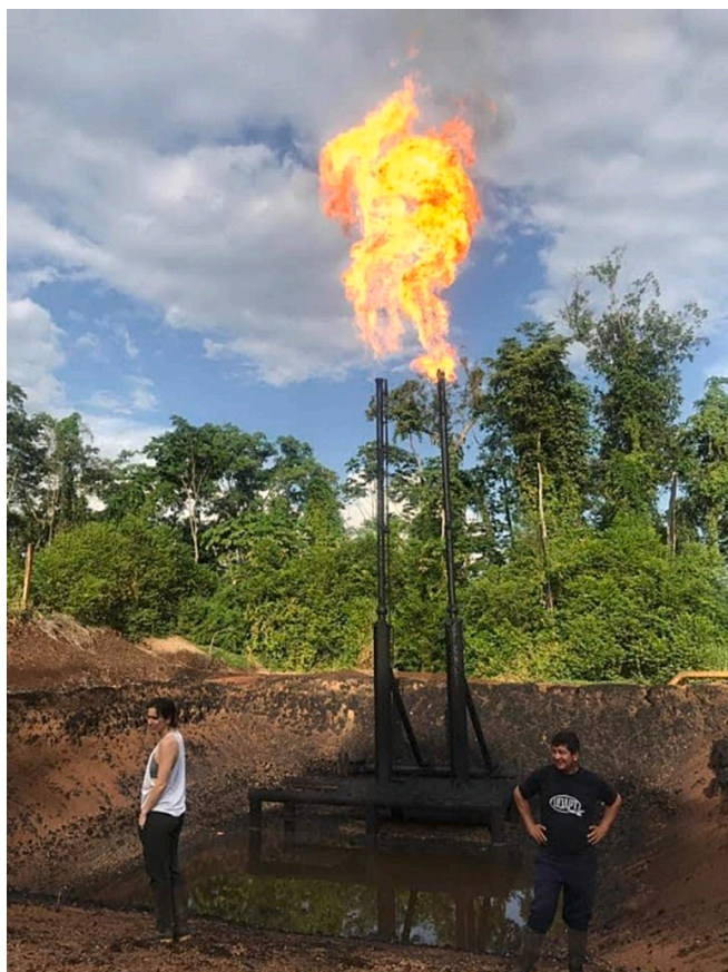
Fig. 1. Waste oil pit and gas flare. Over 1,100 surface waste pits and around 447 gas flares exist within the provinces of Sucumbíos and Orellana in the Ecuadorian Amazon to contain waste oil and production fluids and burn off excess methane [17]. They are significant sources of air, water, and soil pollution.
