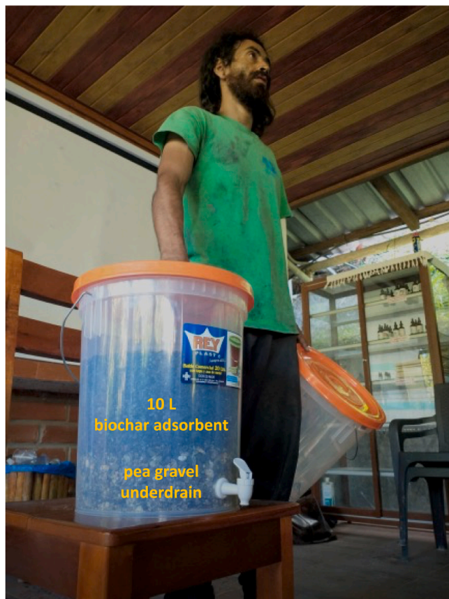
Fig. 5b. Co-author Yepéz demonstrating point-of-use household biochar adsorbent developed through participatory design workshop.
